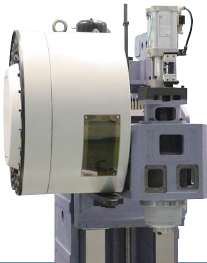
Double protection device in tool magazine
