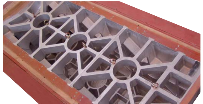
Central-circle and radial-rib Interior of column structure
