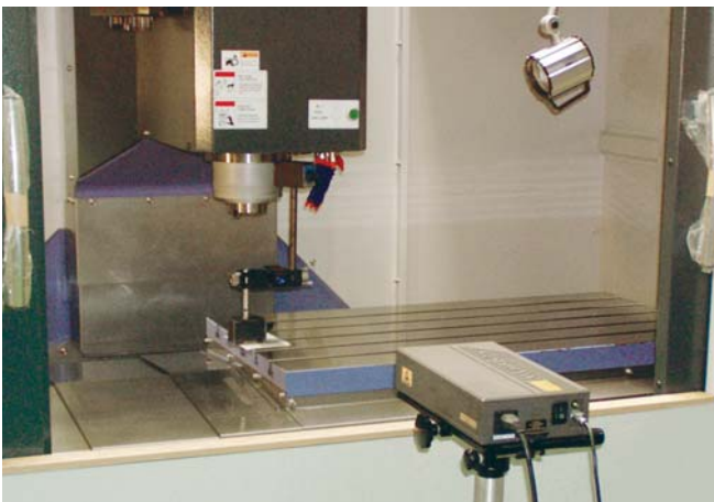
Laser positioning and calibrating
