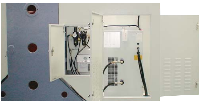
Independent rooms to install pneumatic, lubricating, and cooling systems respectively.
