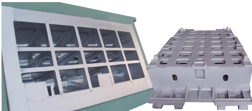
A-shaped rib reinforcement of base structure
